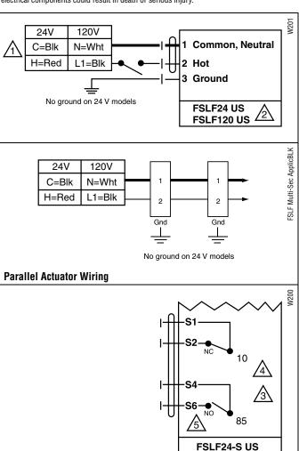
Auxiliary switch wiring for FSLF24-S US, FSLF120-S US
