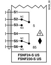
Auxiliary switch wiring for FSNF24-S US, FSNF230-S US
