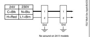
Parallel Actuator Wiring
