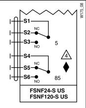
Auxiliary switch wiring for FSNF24-S US, FSNF120-S US
